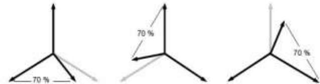
Figure 3b - Phase-to-phase testing on three-phase systems - Acceptable Method 1 phase shift
