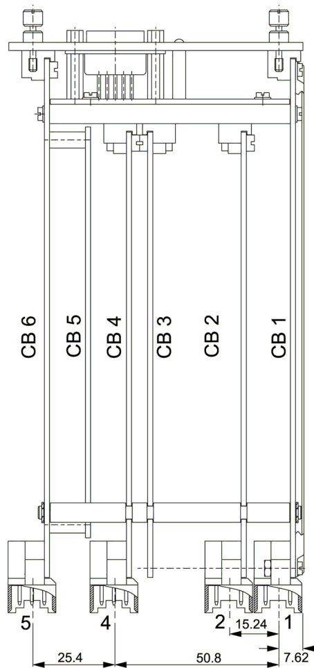
Position of blade connectors and PCBs for feature C10
