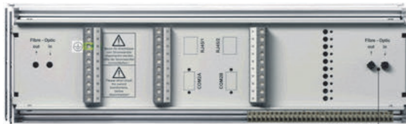
Fibre optic in-/output with ST or FSMA connector
