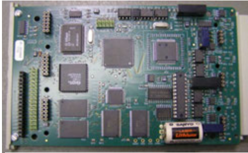
CPU circuit board with soldering battery – plan view
