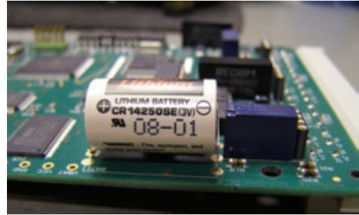
Soldering battery with three soldering lugs
