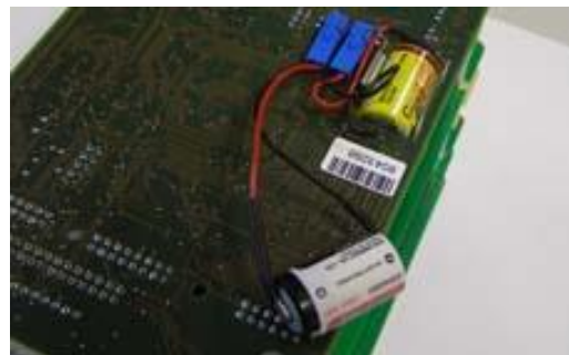
Parallel plugged batteries
