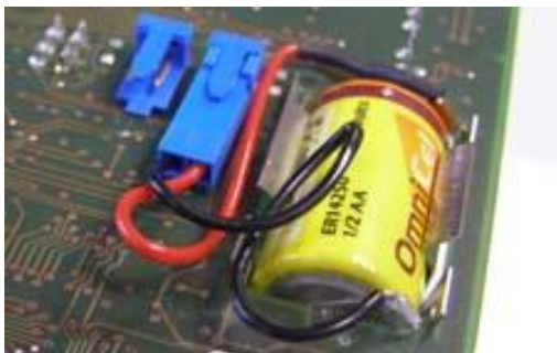
Plug connection points and metal cover on the outside of the printed circuit board
