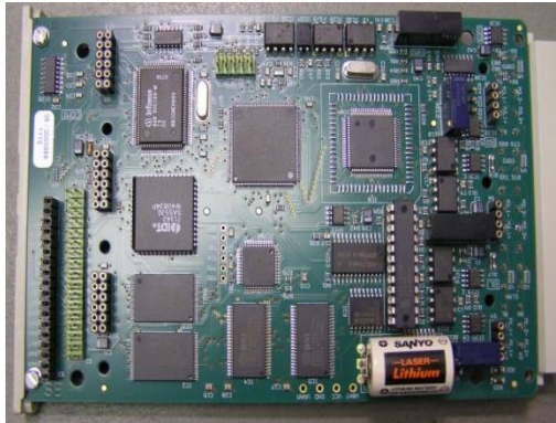
CPU circuit board with soldered battery – plan view
