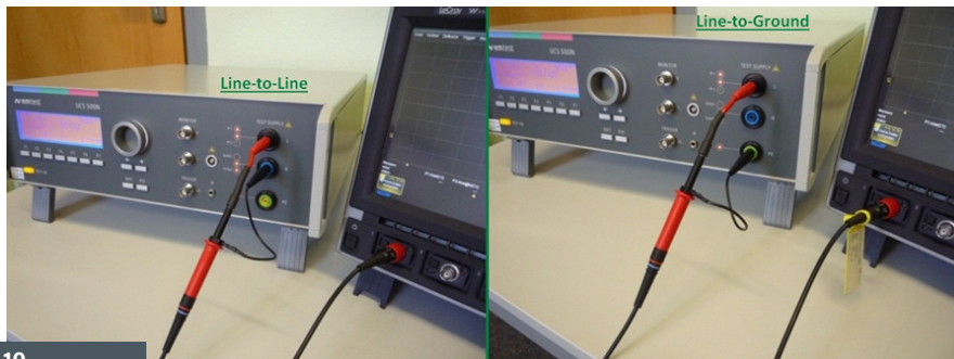
Figure 10 Test set-up to verify open-circuit CGW/CDN system
