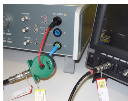
Short circuit current with current probe
