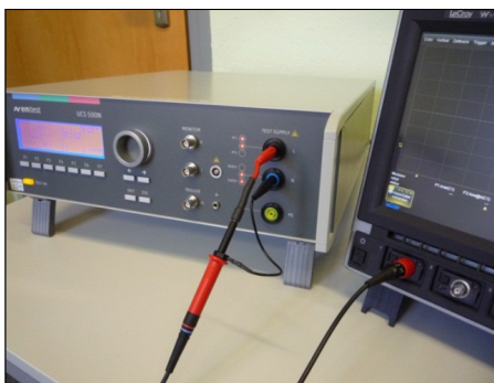
Open circuit voltage with HV-Probe
