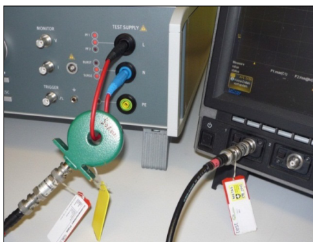
Short circuit current with current probe
