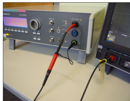
Open circuit voltage with HV-Probe
