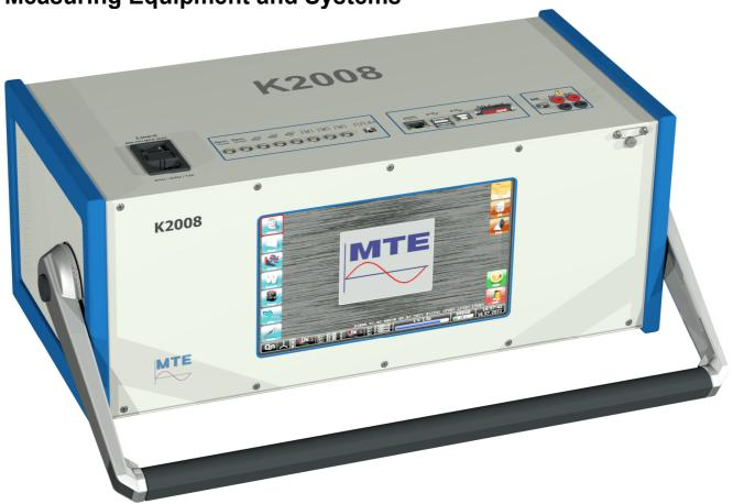
K2008 is a three-phase comparator of accuracy class 0.005 (50ppm) with direct voltage and current inputs. It has been designed for universal laboratory and test applications and is intended for checking and the calibration of reference standards for electrical power and energy. In addition, it can be integrated into meter or reference standard test systems of highest accuracy.
