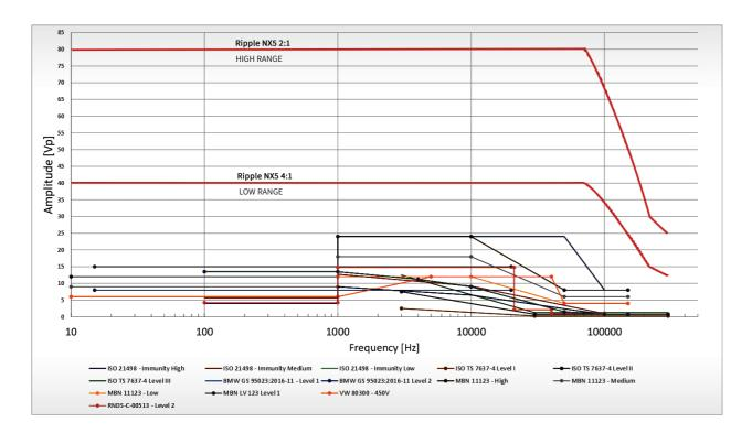
The above graph shows the ripple amplitudes defined by the various standards. The Ripple NX specifications significantly exceed these requirements which provides a wider margin for higher test levels and compensation for voltage drops in connection cables.
