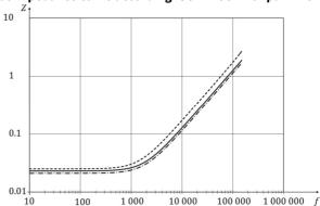
Each set is tuned individually to meet the impedance requirements of ISO 21498-2.
