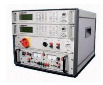
REMAGRAPH®-REMACOMP® combination C - 710 with two electronic fluxmeters EF 5. (The stand-alone computer is not shown.)
