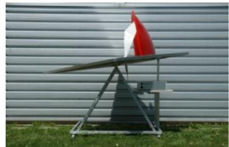
The HIRA180 is an ultra wideband half radiating antenna using a ground plane as an electromagnetic mirror. This antenna produces a very narrow beam in the bore sight direction. The advantage of this construction compared to a full paraboloidal reflector antenna is a better ruggedness, a broader frequency range and an improved return loss.
