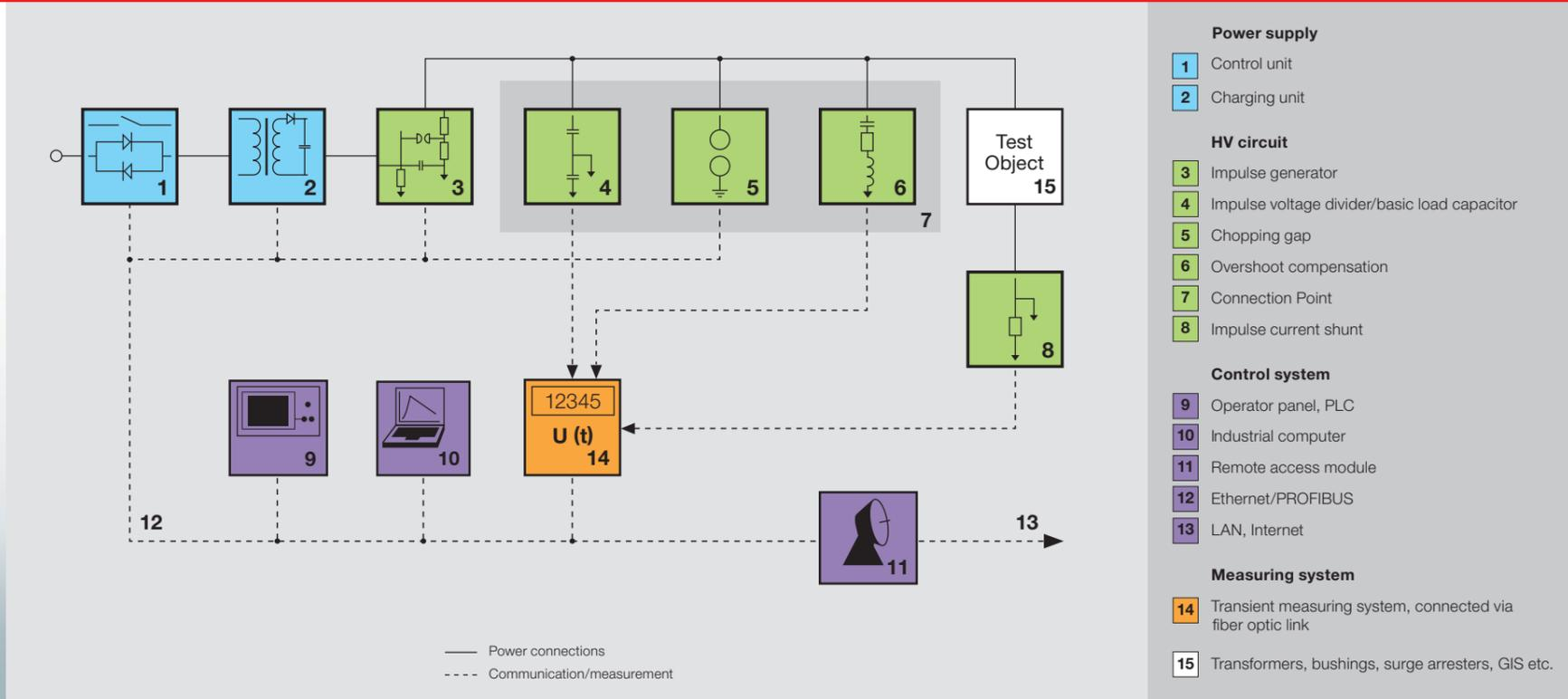
Fig. 3 Block diagram of impulse voltage test system
