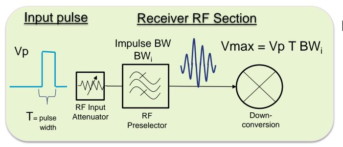
Max Pulse voltage into mixer is proportional to RFPS filter impulse BW (BW<sub>i</sub>)
