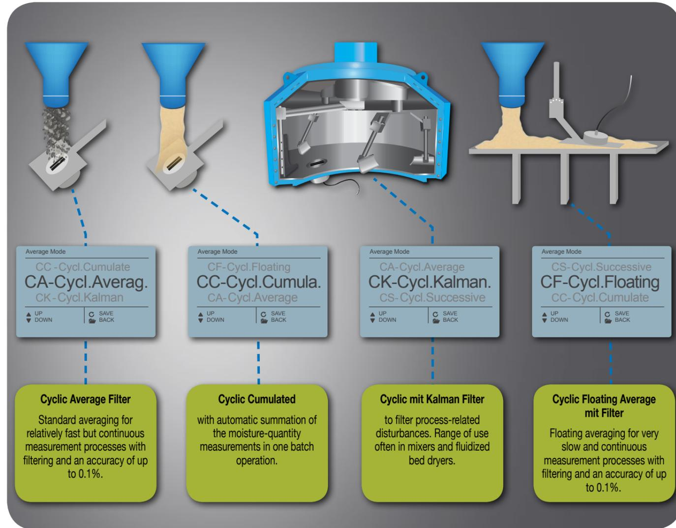
The SONO-probe can be adapted via the SONO-VIEW to the appropriate operating mode like: cyclic measurement, averaging, filtering, cumulating and other powerful operating parameters.
