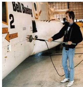
Figure 9 : Example of P-static test
