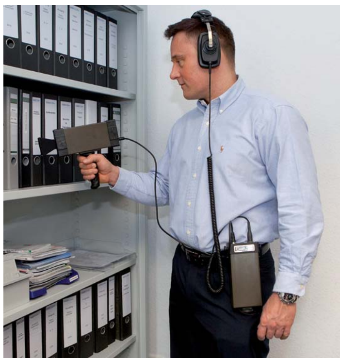
EBEX® 2001 CK for detection of time delay devices in IED and incendiary devices
