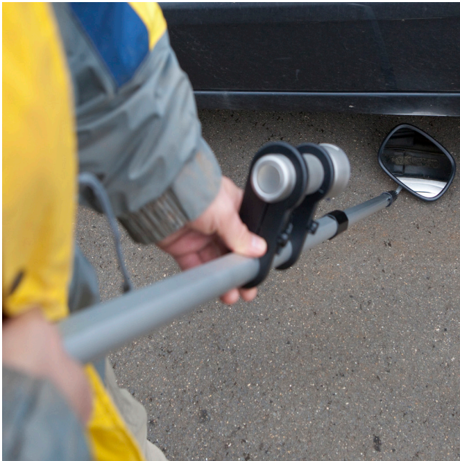
EFIS® 1 inspection mirror with torch
